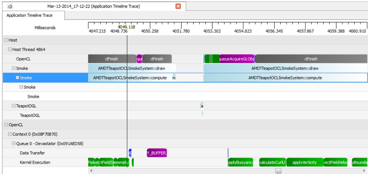
The AMD Developer Tools Activity Logger (AMDTActivityLogger) library provides a simple instrumentation API that can help users to analyze their applications. It allows users to instrument their code with calls to `amdtBeginMarker()` and `amdtEndMarker()`. These calls are then used by CodeXL to annotate the application's timeline in a hierarchical way.
